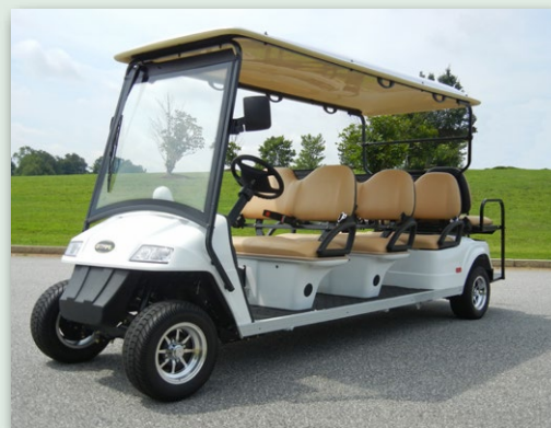
Solid front bumper, rack and pinion steering
