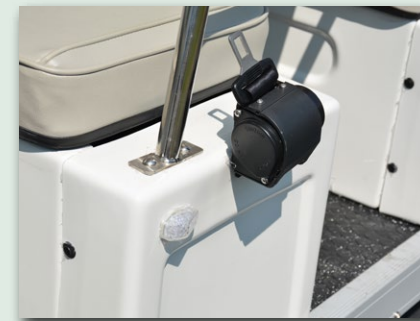
LED side lights and seat belts for safety
